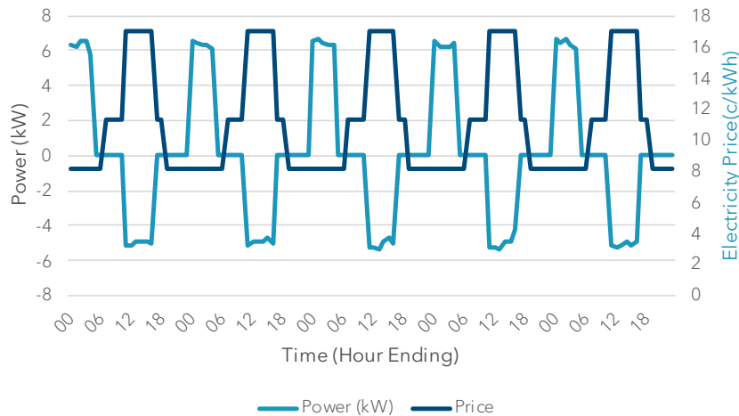
Figure 14. Power transfer against electricity prices for arbitrage test.
